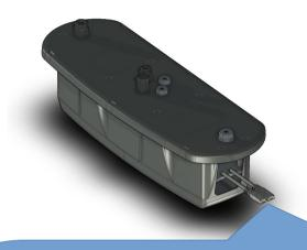
Route the two 2m Ethernet cables from the port hatch assembly to the stbd hatch assembly through the BlueBoat crosstube. Inside the stbd hatch assembly connect one Ethernet cable to the Rpi and the other to the BlueBoat router using the Ethernet coupler provided. Refer to the BlueBoat integration guide for more details.
